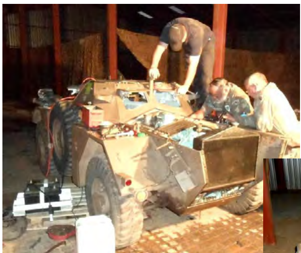
Below The pressure was really on these Armour Museum volunteers to make an emergency over night engine change on this Ferret Scout car . Enthusiasts were invited to visit the Sandstone workshops to inspect the proceedings . Although busy the mechanics still had time to tell me the original engine was malfunctioning due to the oil and petrol being mixed up .
