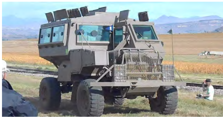
Right Saracen Armoured Personnel Carrier of British origin using Rolls Royce straight 8 petrol engine but South African modified with larger wheels suit local conditions, 1950s to 1970s . These were superseded by the South African made Buffel mine proofed troop carrier shown Below
