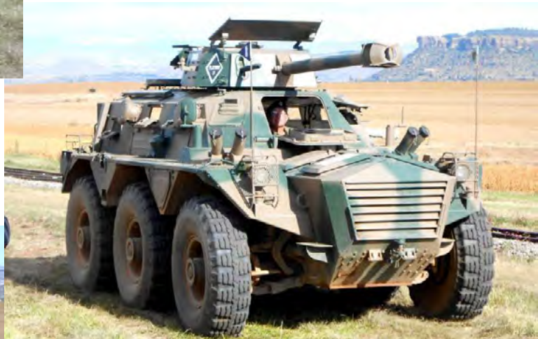
Right Saracen Armoured Personnel Carrier of British origin using Rolls Royce straight 8 petrol engine but South African modified with larger wheels suit local conditions, 1950s to 1970s . These were superseded by the South African made Buffel mine proofed troop carrier shown Below
