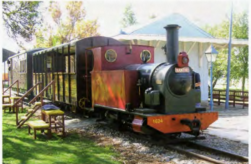
XANTHE 0-4-0T Avonside 1624 of 1912 at Sandstone Estate. Due to demand many trains scheduled to be hauled by small locomotives were hauled by NGG Garratts. Photo: Wendy Black
