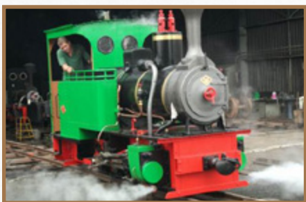
O & K 12493 undertakes a steam test after restoration prior to leaving for Germany.
