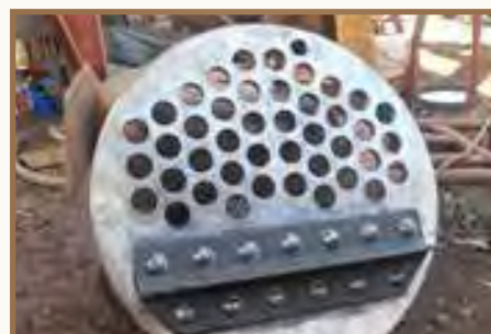
The new tube plate which has been fabricated
