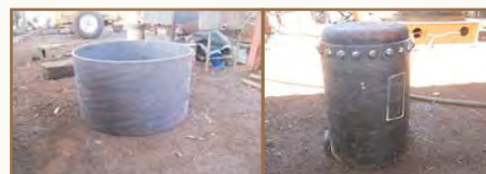
The smoke box outer wrapper The new dome partly complete
