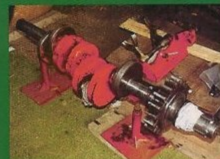
Having been lifted out of its bearings, the crankshaft is on the floor with part of its gear change mechanism.
