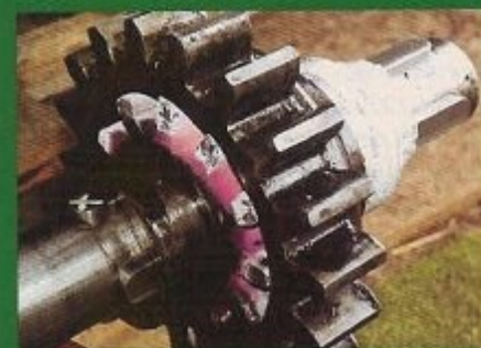
The four keys were a poor fit on inspection and, after re-working by Leek's, they were made good.
