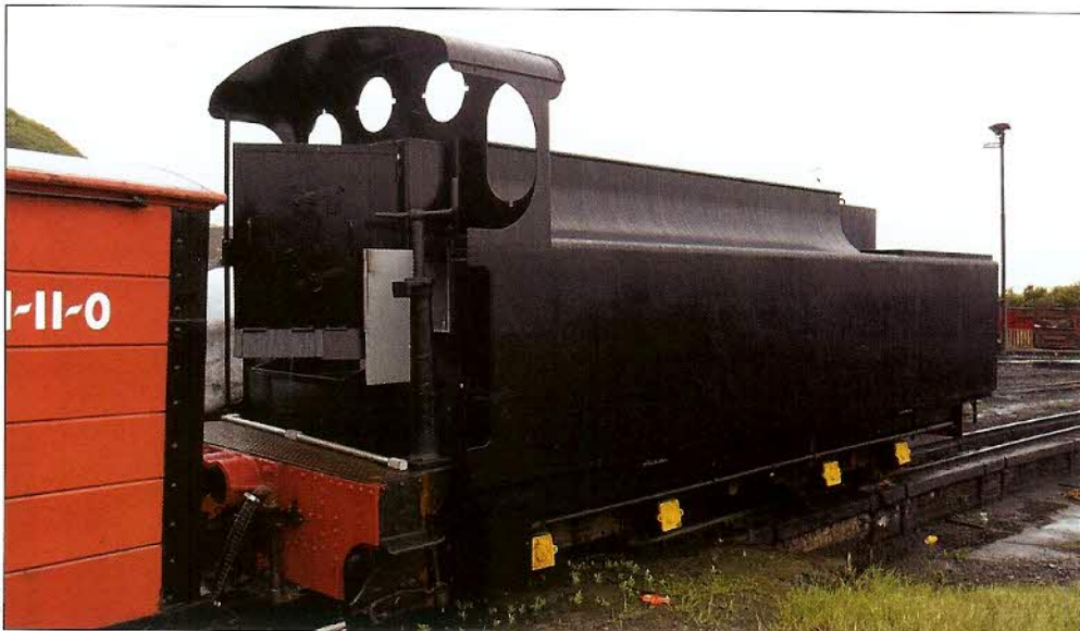
Below: Mounted temporarily on no 133's underframe, the new tender body was on show at Porthmadog in summer 2012. Both photos: Andie Shaw
