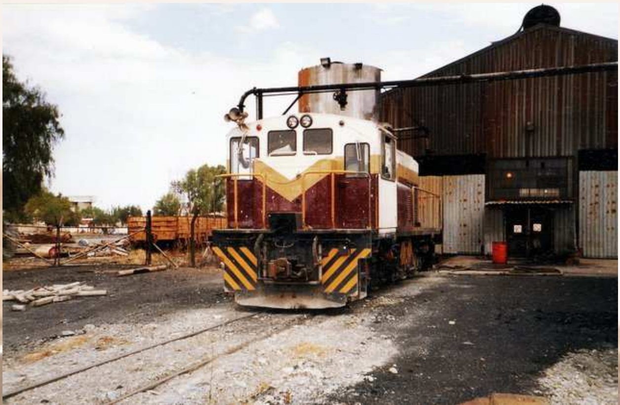
Below: Number 2 at SANRASM, the main frames were cut to get the axle boxes out and she now is doomed to. This is the very end of the 16CR's of St Helena, Sandstone Estates now have the only serviceable Class 16CR from St Helena Gold Mines.
