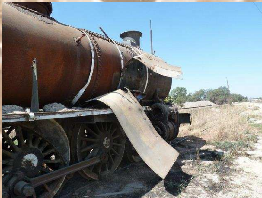
Below: Number 2 at SANRASM, the main frames were cut to get the axle boxes out and she now is doomed to. This is the very end of the 16CR's of St Helena, Sandstone Estates now have the only serviceable Class 16CR from St Helena Gold Mines.
