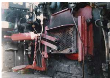
The modified firebox doors
