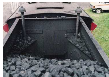
The coal bunker of 141
