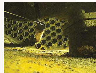
The boiler tube, which initially failed on a day-trip to Maraisburg, is blocked by the brake ejector exhaust while being withdrawn from the front tube plate. Upon closer inspection facilitated by the one tube being withdrawn – other boiler tubes were found to be wasted as well.
