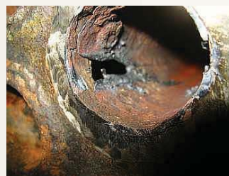
Here is a wasted boiler tube in the process of removal. The visible hole has just been cut by a torch to collapse the end of the tube to draw it out. However, the wasting and corrosion is clearly visible at the 10 – 11 o' clock position. Note the tube beading has already been ground off in this picture.
