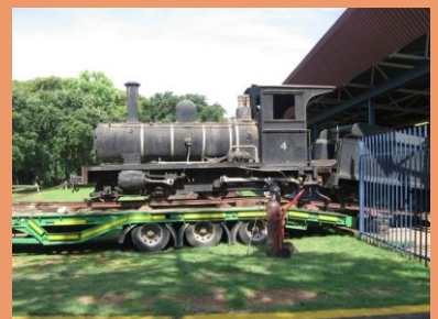
The air in the low-bed's air cushion suspension can be released allowing the deck to drop nearer to the ground
