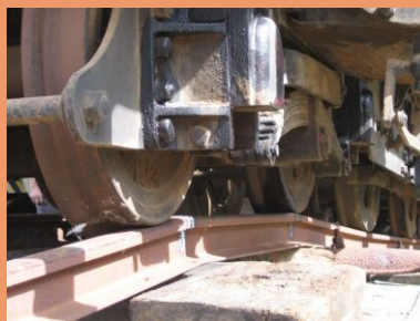
A close-up view showing the location of the rail head cut-outs
