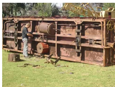
The B-bogie bodies are lifted from the bogies for attention to the underside and then refitted on to the bogies.
