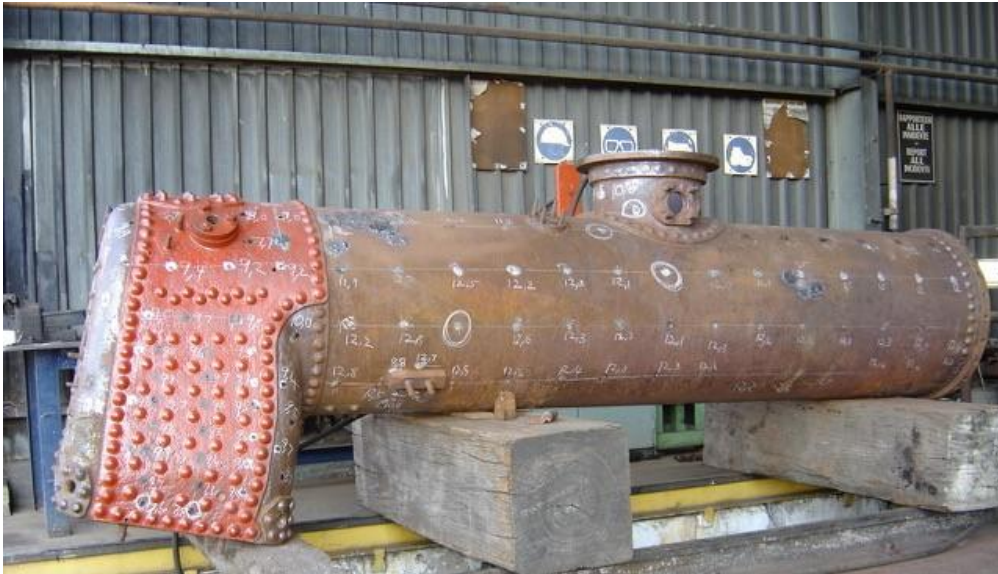
The old boiler of the Feldbahn removed from the frames for inspection.
