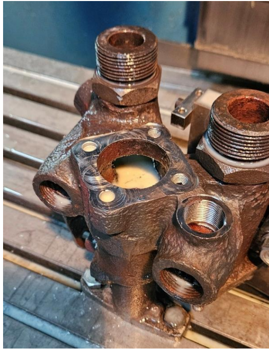
The regulator bolts drilled out and the seats machined.
