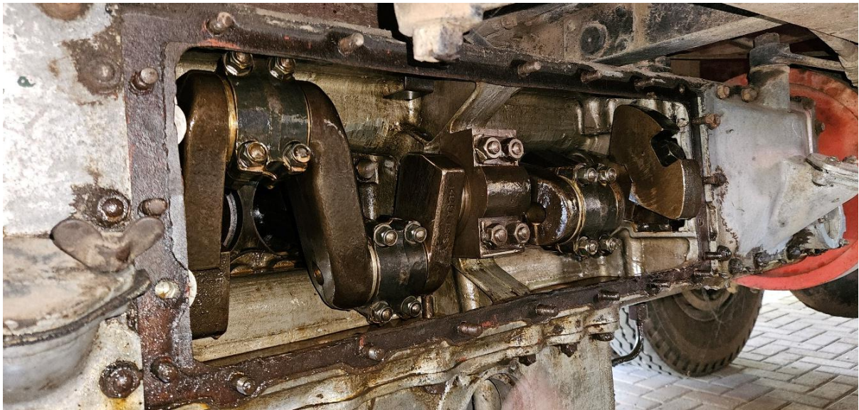
The crankshaft of the Sentinel showing the engine's similarity to a normal internal combustion engine.
